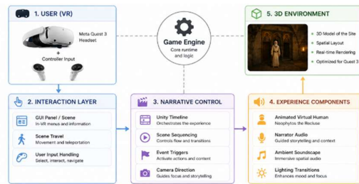
Figure 4: The layered architecture of the immersive VR experience developed in Unity for Meta Quest 3.
