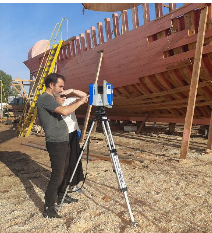
Terrestrial Laser Scanning at the shipyard
