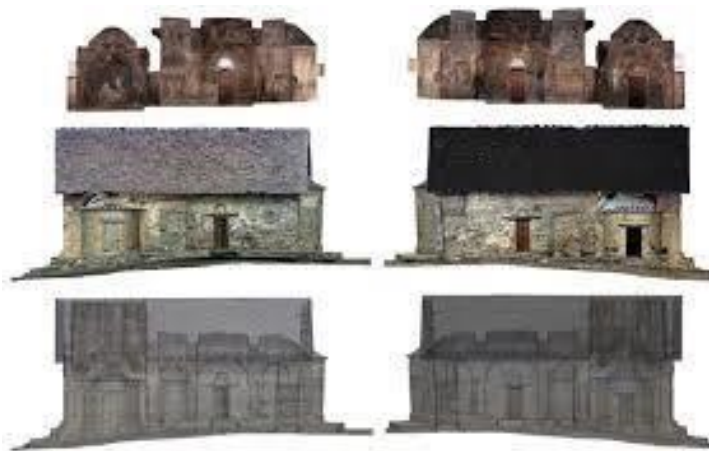
Figure 16: The 3D model of ASINOU and its corresponding Orthophotos from the exterior and the interior.
