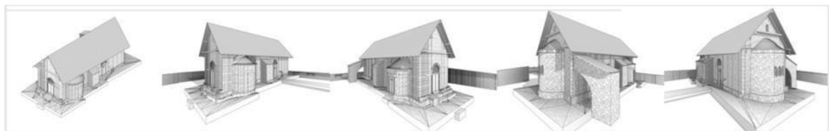
Figure 15: The BIM representation of the exterior of the ASINOU monument in Revit.
