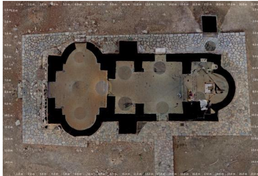
Figure 9: The 3D laser positions for the 2D and 3D holistic documentation of ASINOU monument.
