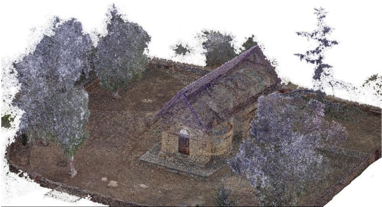
Figure 10: The final merged point clouds from all the different laser 3D data acquisitions.
