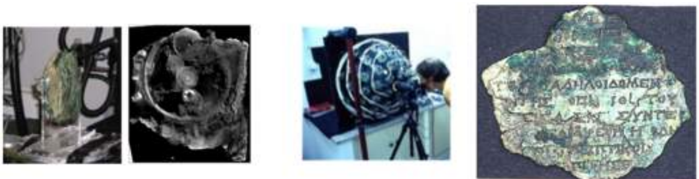
Figure 3. X-ray tomography of the fragment A by Roger Hadland (left) and investigation of the fragment 19 using the PTM Dome technique by Tom Malzbender and Dan Gelb (right).
