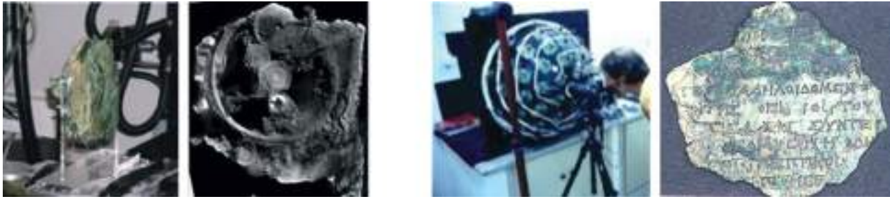
Figure 22. X-ray tomography of the fragment A by Roger Hadland (left) and investigation of the fragment 19 using the PTM Dome technique by Tom Malzbender and Dan Gelb (right).
