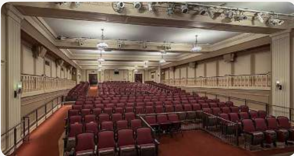
"Reconfigured seating accommodates wheelchairs in front and middle via lift and ramps, and rear from main doors, AV hidden behind beams." Photo by Mark Ballogg
