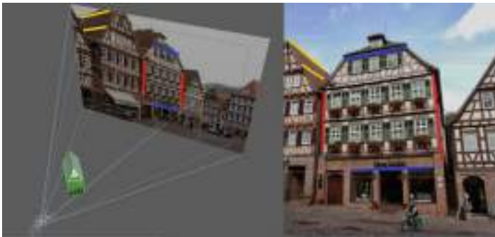
Fig. 14. Set-up with the calculated camera position and the 3D Model of Hermann Hesses Birthplace (Figure created by the authors and cited in [29]).
