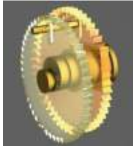
Fig. 20. The pin-and-slot mechanism [20].
