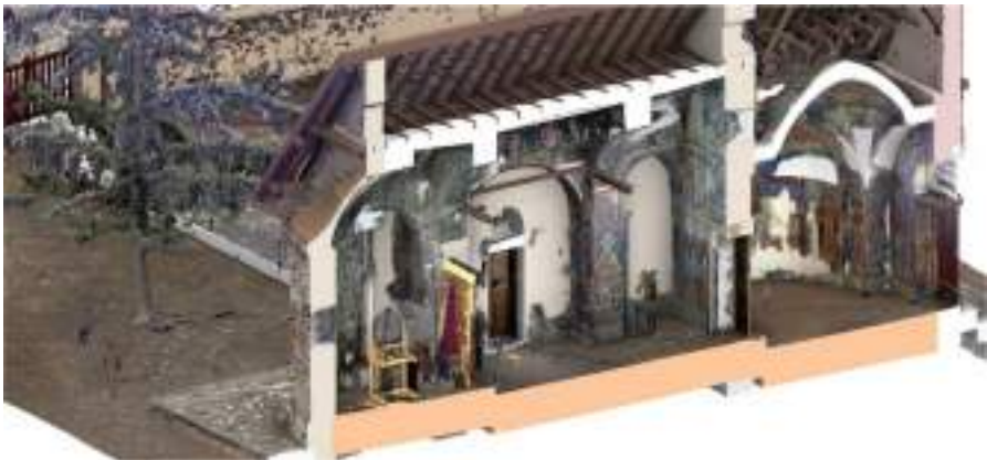
Fig. 3. 3D model elevation, generated by point cloud (Color figure online)
