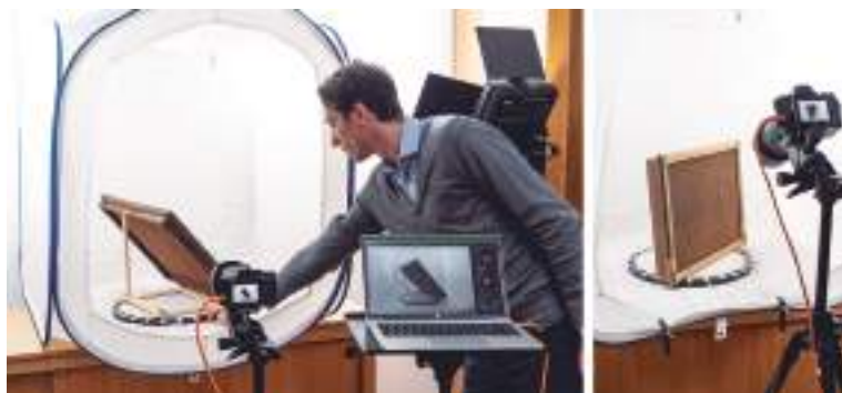
Figure 51. 3D digitisation process using photogrammetry at Museo della Carta
