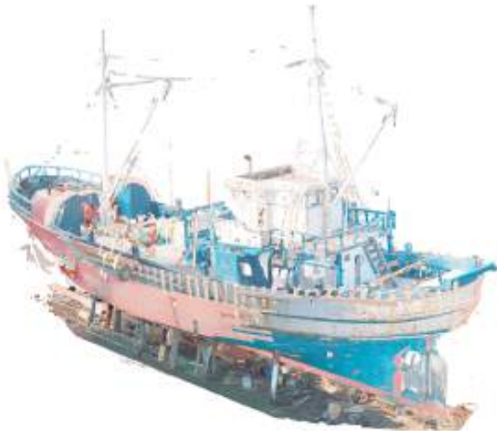
Figure 25. Aligned TLS and Photogrammetric point clouds
