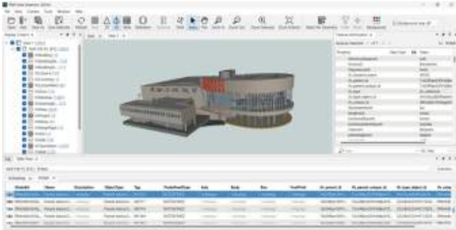
Fig. 4. Pampulha Art Museum model visualized in the Data Inspector FME with missing axis, body, and description information.
