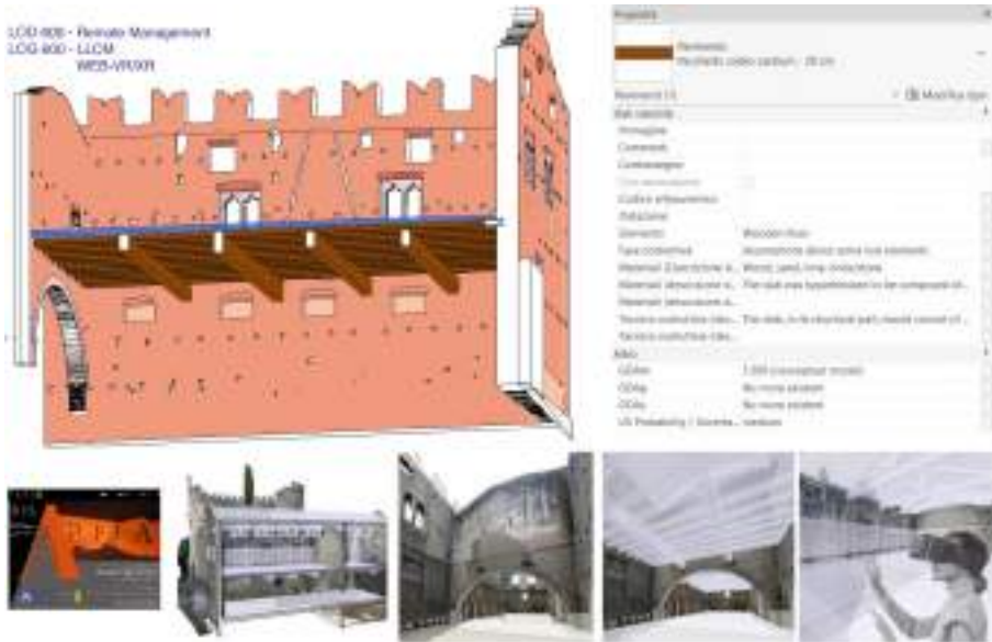
Fig. 5. Construction phases progressively embedded into informative models supporting Virtual Reality (LOG600): the HBIM ‘Fireplace’ Hall at the 1 st floor (Upper). The reconstruction of the no longer existent wooden floor (GOAm 200) included in the HBIM Paradata. The immersive exhibition opened to public on Dec 2023 (Below), (Courtesy of ABCLab-GIcarus and PAAA ©).
