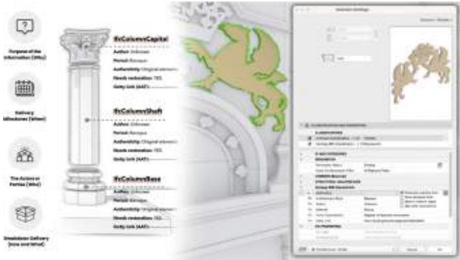
Fig. 2. Level of Information Need and classification assessment in BIM software of choice – Graphisoft Archicad.
