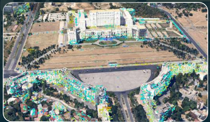
Satellite radar scans show various points on and around the Palace that are slightly rising in blue or sinking in yellow/orange (source: Terrasigna)
