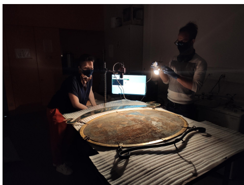
Photo (left): Set-up of the VNIR hyperspectral camera on an oil-painted metal shop sign «Lido 1870» (ML/2019/0830, Musée du Léman à Nyon, Switzerland).
