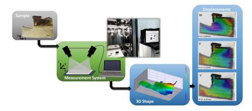
Photo: Example of a historical sample, measuring system and output quantities from a 3D DIC measurement. The sample is subjected to humidity fluctuations which result in the formation of displacements and change of its shape.
