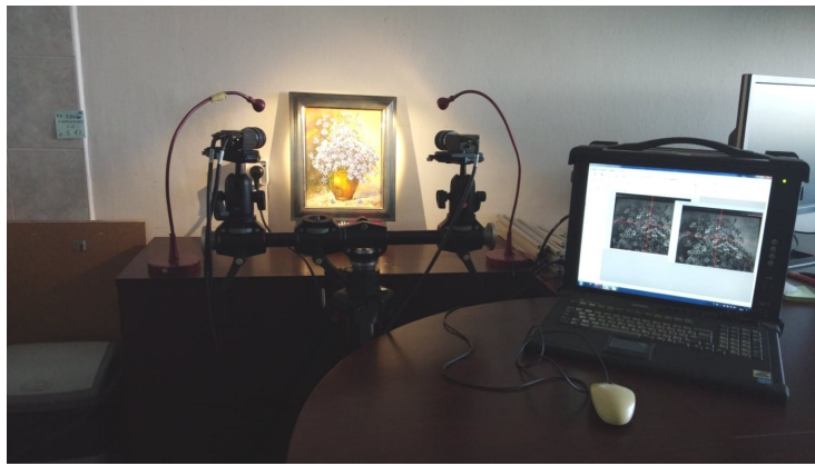
Photo: Monitoring the object's surface with Digital Image Correlation Setup (Sunita Saha)
