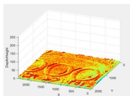
*Photo: Basic 3D depth map of coin, used for further digitization methods*
